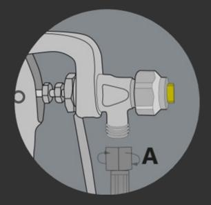
Once you're ready for work to commence open the canistervalve turning it clockwise by hand.
